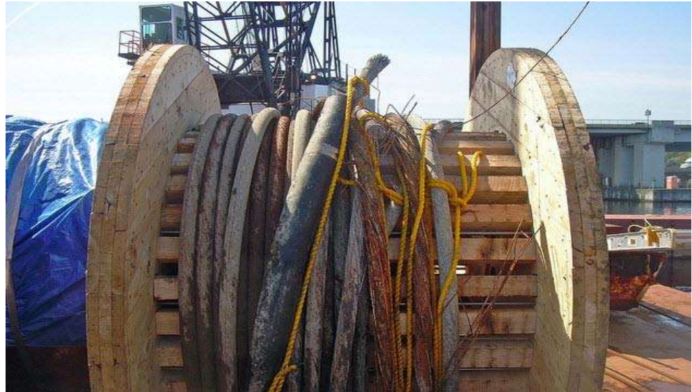
Figure 16.3.18 Frayed Cables Removed from a Floating Bridge
